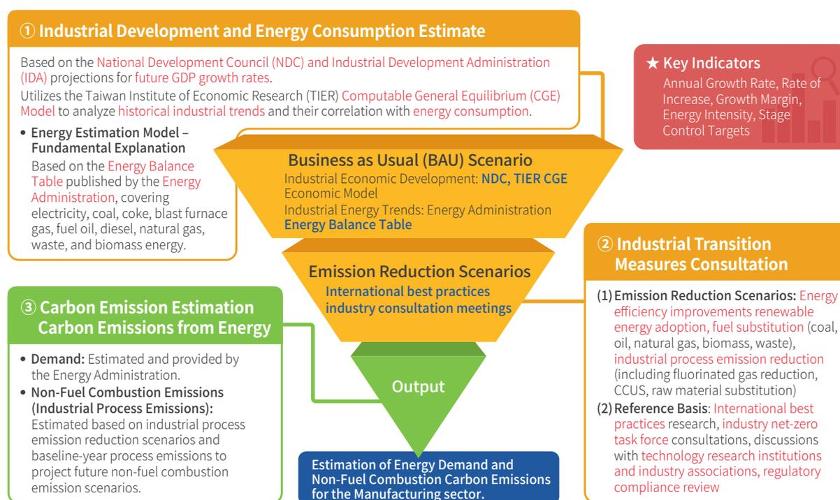
Figure 4.3.2-2. Flowchart for Estimating Manufacturing Sector's Greenhouse Gas Emissions Trend
