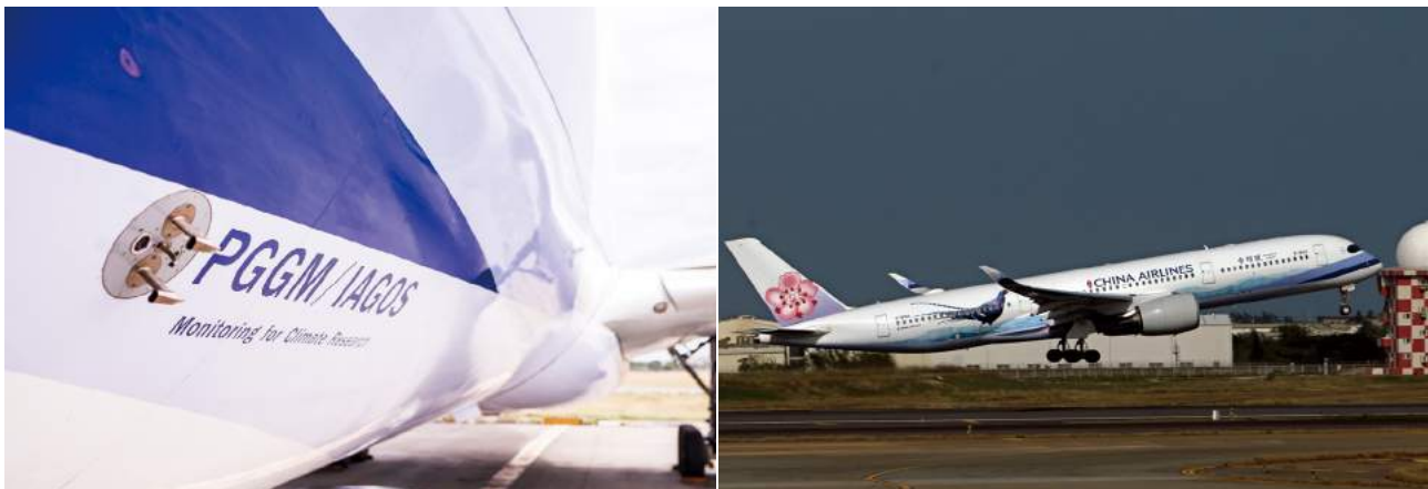
Figure 8.4.2 China Airlines loads the global observing instrument system on the A340-300 passenger aircraft
